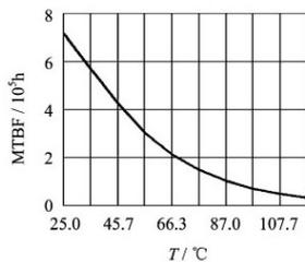
Fig.5 MTBF-temperature curve
