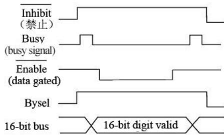
Fig. 5 Time sequence of 16-bit bus transfer
