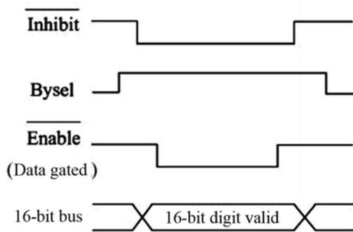
Fig. 3 Time sequence chart for 16-bit bus transfer
