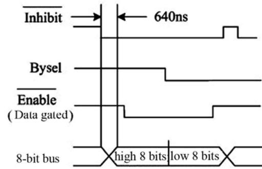
Fig. 4 Time sequence chart for 8-bit bus transfer
