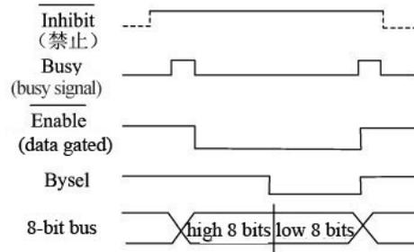
Fig. 6 Time sequence of 8-bit bus transfer
