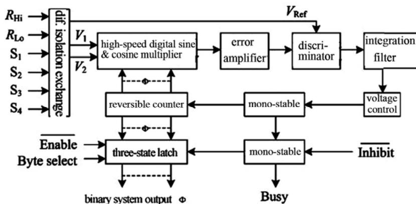
Fig.2 Block diagram of operating principle
