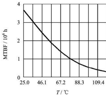
Fig.7 MTBF-Temperature Curve
