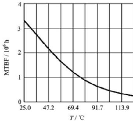
Fig. 4 MTBF-temperature curve
