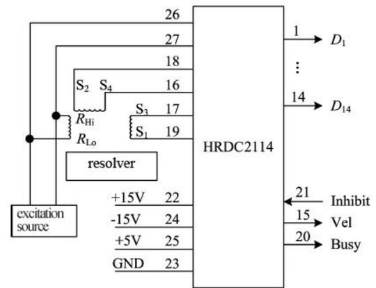
Fig.6 Connecting diagram of typical application
