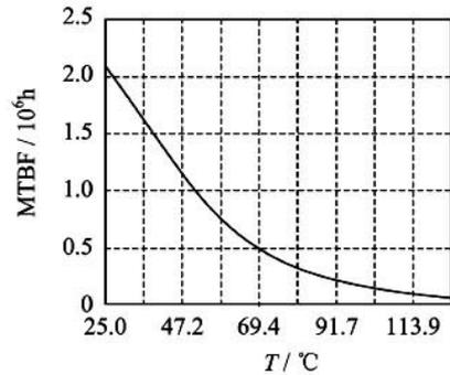
Fig. 3 MTBF-temperature curve
