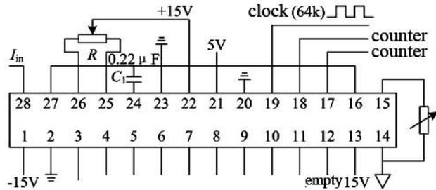
Fig. 5 Connection diagram for typical application
