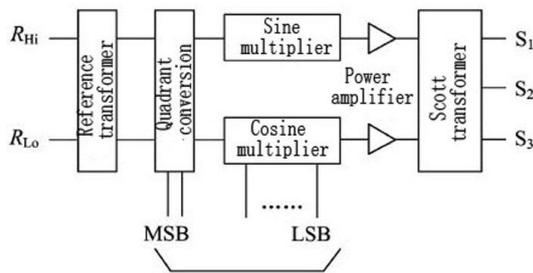
Fig.2 Schematic diagram of MDSC converter
