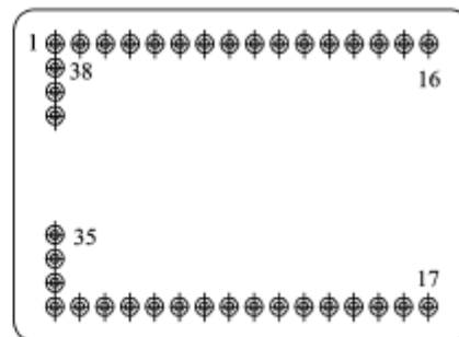
Figure 5 Pin out bottom view
